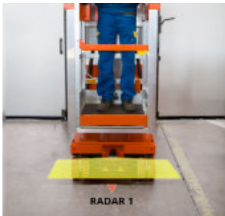
RADAR1 Frontal Anti-collision Radar System
