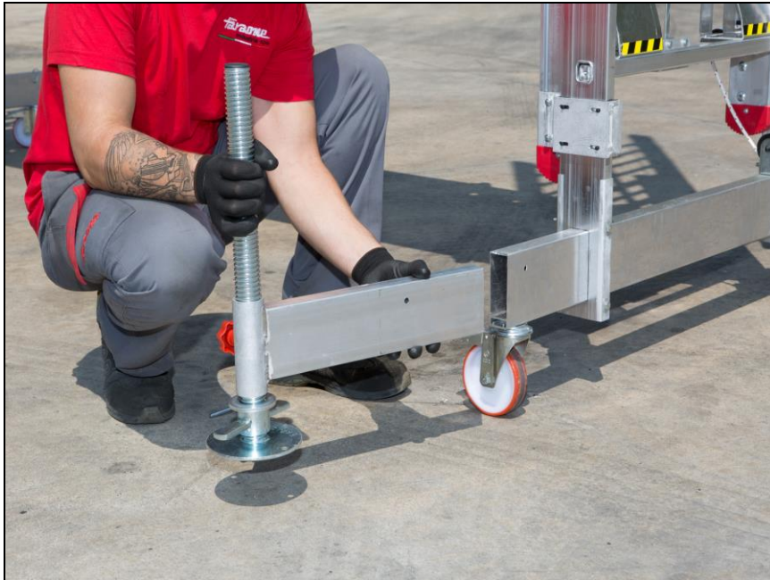
Fig.1: Insertion of outrigger bases
