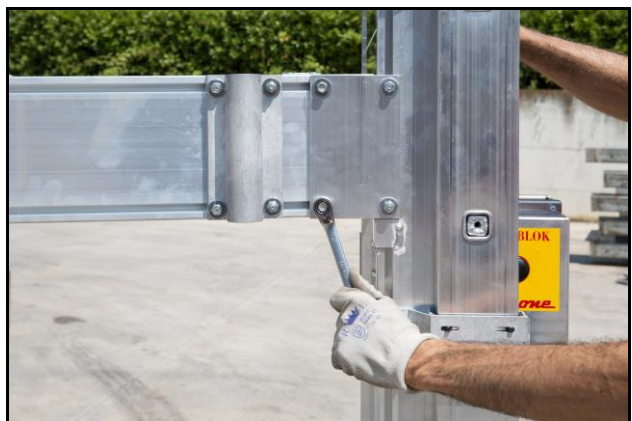
Fig.5: Deck attachment plate detail
