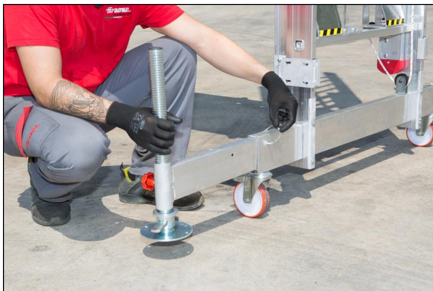
Fig.2: Locking of outrigger bases
