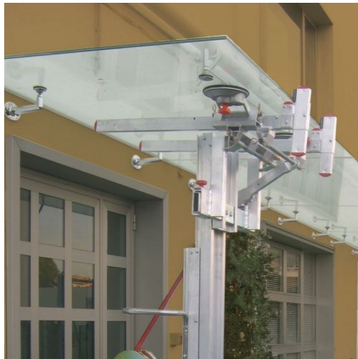
Suction cup kit with swivelling support for lifting glazed panels.
